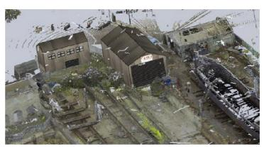
A close up of EAPL's proposed buildings in situ alongside as-built data from the point cloud.
