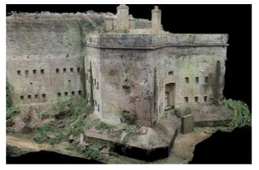
Part of OmegaGeo's point cloud of Leeds Castle, captured using a mixture of terrestrial, aerial and water-based scans. The point cloud was animated using Veesus Arena4D's high-definition point cloud animation functionality.
